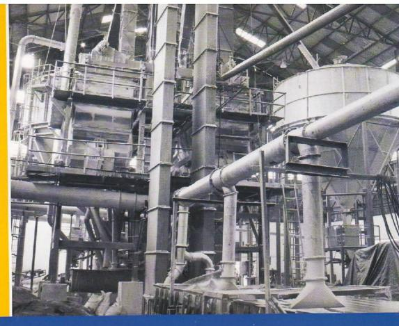
AIROCHEM has manufactured various types of sugar dust collector systems and supplied to many sugar mills in India and abroad.
