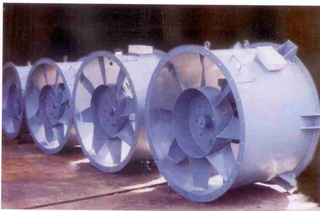
Axial Flow fan for Cochin Shipyard Ltd. for Ship Ventilation.
