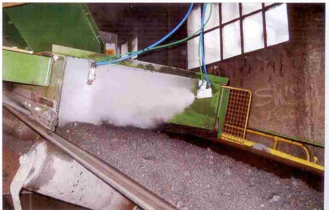
Dry Fog Nozzle placement & flow of material.
